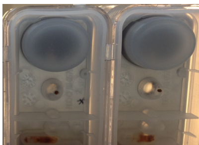
Figure 1: Picture of bead pellet in PCR well after cassette processing has completed.
