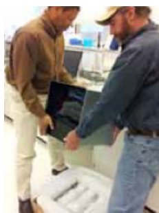
16) Using your legs, lift the unit straight up and out of the lower foam and box
